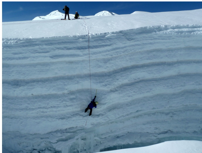
Figure 3.1: Measurement of snow and firn layers on Suyuparina glacier, southern Peru. Credits: photo by Christian Huggel .
