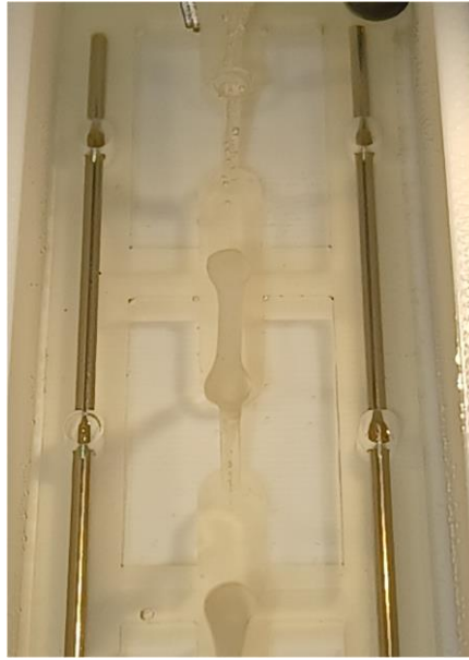
Figure 26. A custom 3D printed chamber used to measure action potentials in EHTs. (Photo by: Flavien Charpentier)
