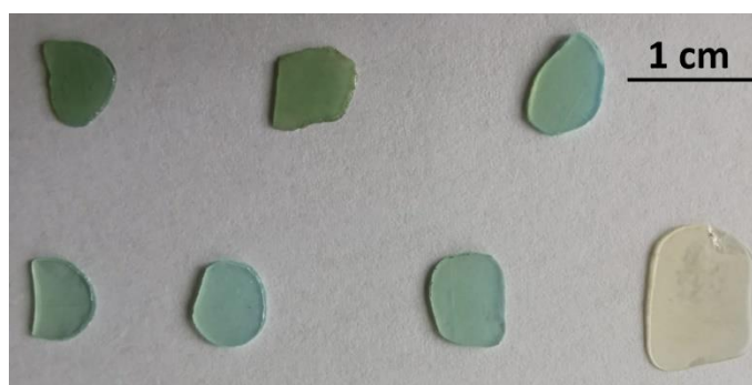
Figure 3. 3: Image of the microplastic pellets obtained by the moulding of metal sorbed nanoplastics model materials.
