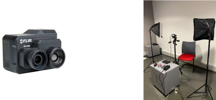
Figure 4.1: The material for the LVT Face Dataset collection is presented: Flir Duo R camera (left) and acquisition setup (right).
