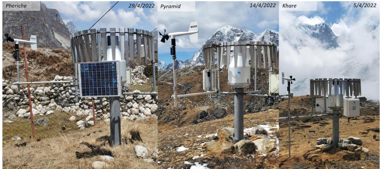
Figure 3.4. Photos of Pheriche, Pyramid, and Khare precipitation gauges (Geonor), along with the date of the photo taken.
