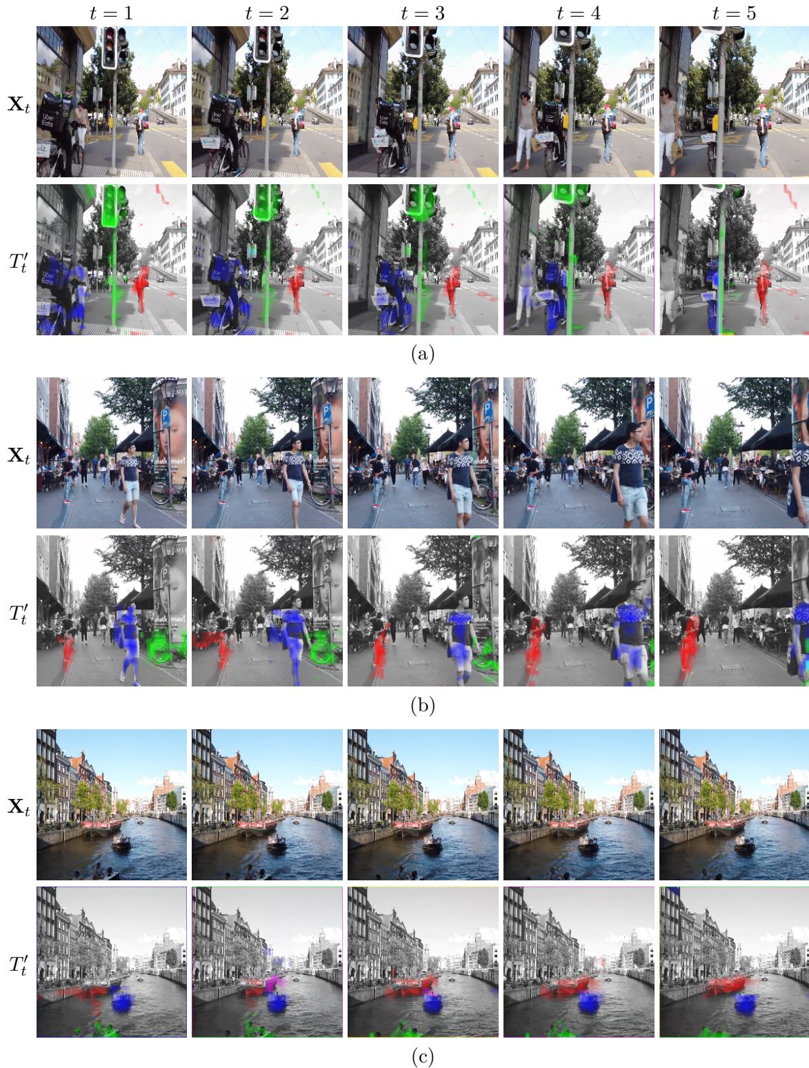
Figure 6.5 – For each input frame X_t of a video clip, refined cross-attention map T'_t \in \mathbb{R}^{k \times n} (6.6), using Sinkhorn-Knopp. For each object, one row of T'_t is reshaped as h/p \times w/p and upsampled to an h \times w attention map overlaid on the input frame for k = 3 objects encoded in blue, red and green channel. T'_t yields three well separated objects shown in blue, red and green.
