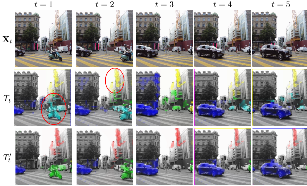
Figure 6.4 – For each input frame t of a video clip (top), cross-attention map T_t \in \mathbb{R}^{k \times n} (6.3) (middle) and refined cross-attention map T'_t \in \mathbb{R}^{k \times n} (6.6) (bottom), using Sinkhorn-Knopp algorithm. For each object, one row of T_t or T'_t is reshaped as h/p \times w/p and upsampled to an h \times w attention map overlaid on the input frame for k = 3 objects encoded in blue, red and green channel. Mixed colors yellow and cyan for T_t (middle, in red circle) indicate spatial overlap of two objects, while T'_t (bottom) yields three well separated objects shown in primary colors blue, red and green.
