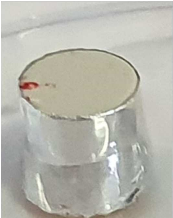
Figure 3.18: Weathering in the presence of NaCl: (A) photographs of the 2X2cm sample before weathering (A).1 and after 3 cycles of weathering (A).2 (courtesy of Rozeline Wijnhorst). (B) photographs of the cylindrical sample before weathering (B).1 and after 4 cycles of weathering (B).2.
