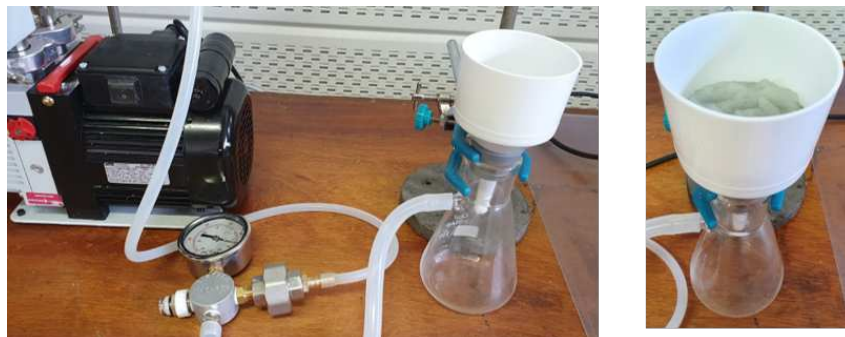
Figure 4: Vacuum evacuation of epoxy
