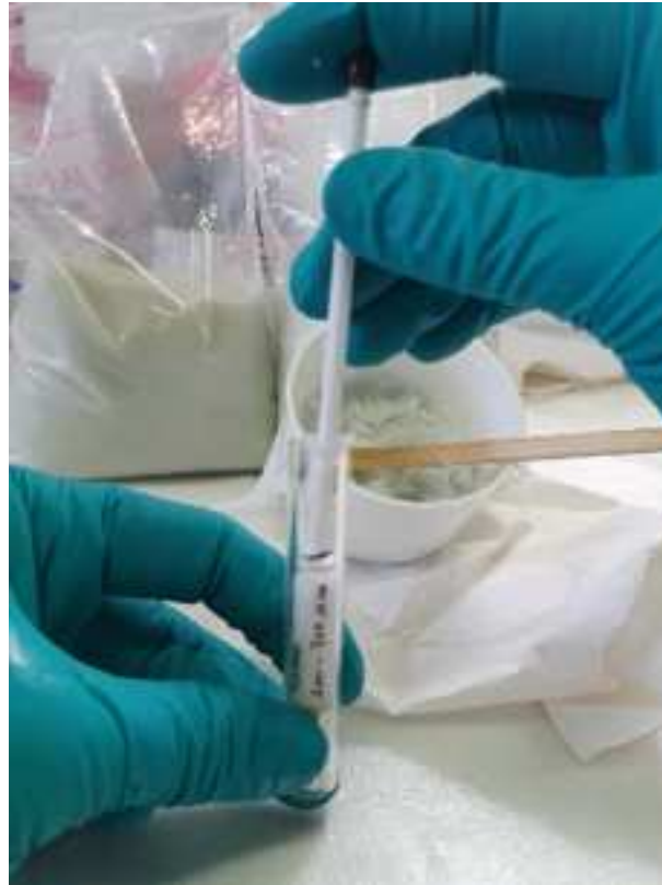
Figure 5: Compaction of the mixture granular media - epoxy into a mold
