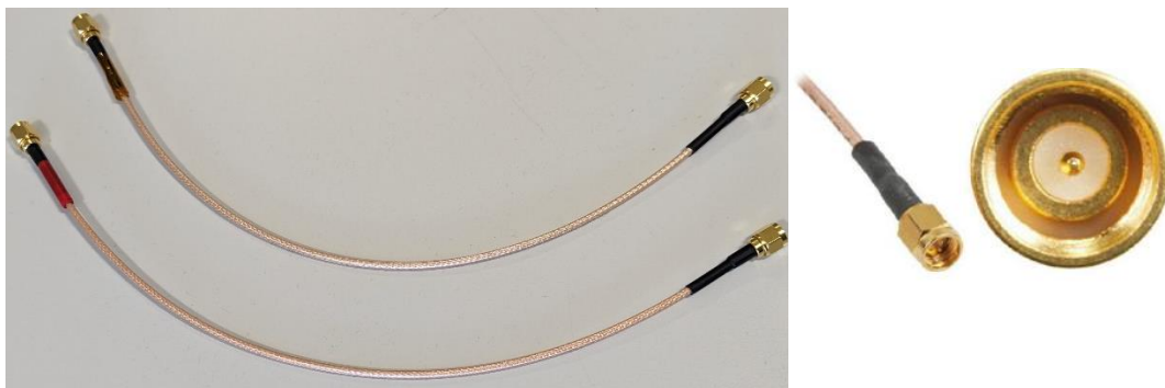
Appendix 4-4. Coaxial cables - SMA with male contact, L=304.8 mm, characteristic impedance is 50 ohms
