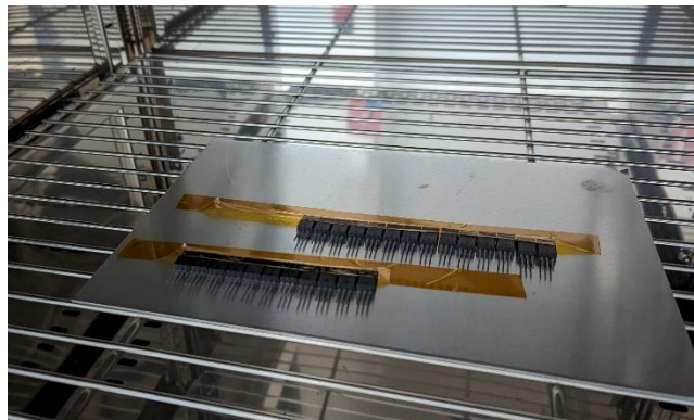
Figure 175: Discrete power samples placed inside climatic chamber
