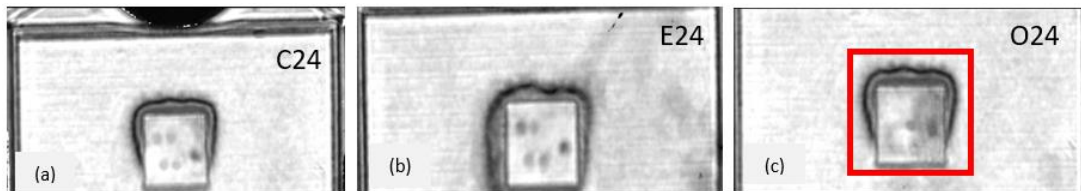
Figure 170: SAM images highlighting bond wire connection after aging of three devices of Group2
