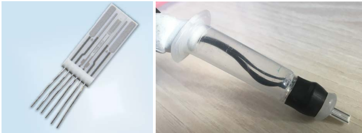
Figure 2.17 – Left: Photo of the IST LFS1K0 conductivity sensor. Dimensions of the ceramic substrate are 12.9x5.5m. Courtesy of IST company. Right: photo of the sensor after marinization for laboratory testing. The Pt-Ni wires are soldered to a Molex Picoblade connector and inserted into a 5mL plastic syringe with its plunger removed. Hot-glue and heatshrink tube is added at the tip of the syringe to make the sensor waterproof.
