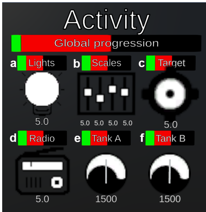
Figure 3.6 – Status of MATB-II tasks: SYSMON (a,b), TRACK (c), COMM (d), and RESMAN(e,f).
