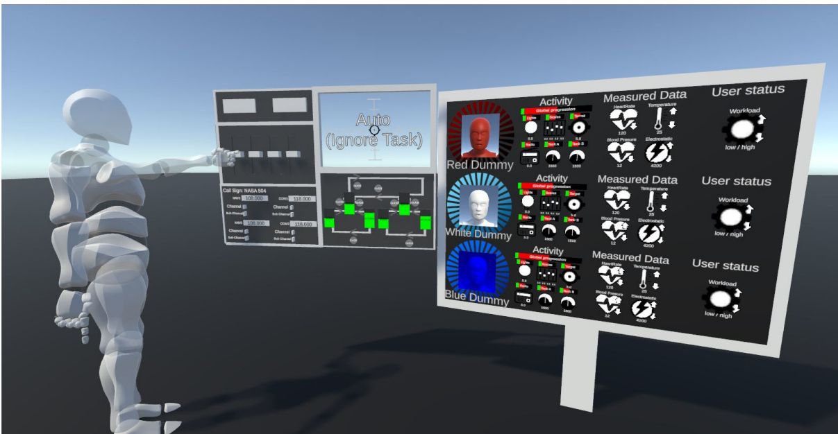
Figure 3.3 – Aggregative: Panel, the information is in a fixed place in the workspace.
