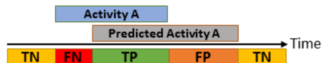
Figure 4.12: An example TS-CM calculation after composing the classifier results. (abbr. T=True, F=False, P=Positive, N=Negative)
