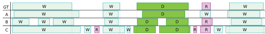
Figure 5.3: Sample ground truth with multiple classes and three different predictions. All these predictions have similar accuracy but the types of their errors are different [Min+06].
