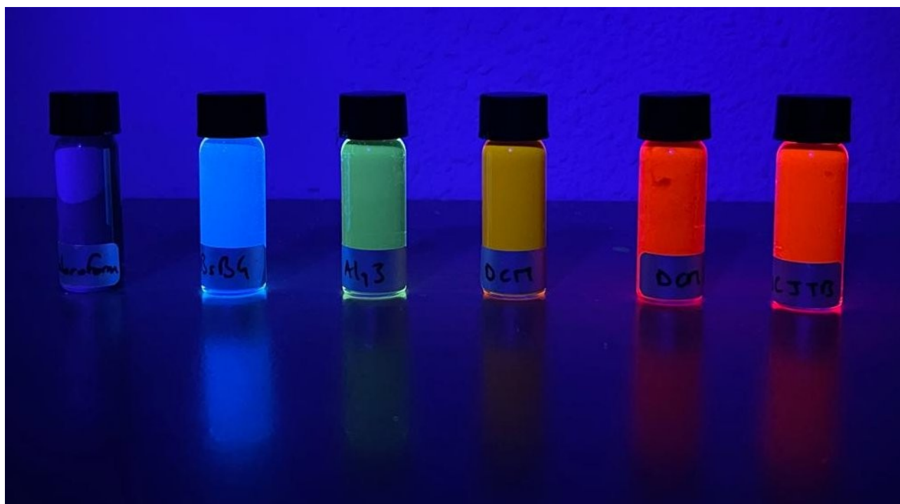
Figure. II.18: Photoluminescence of 5 organic compounds diluted in chloroform (1 \mu mol/ml), from left to right chloroform, BsB-Cz, Alq 3 Alq 3 , DCM, DCM2, DCJTb exposed to UV light from a LED emitting at 405nm.
