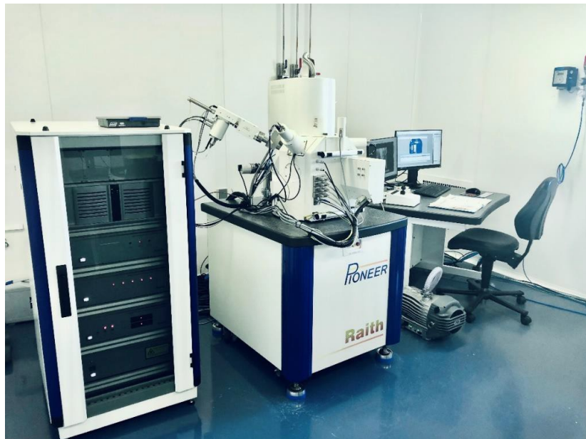
Figure III.19: Photo of the Raith scanning electronic lithography system in C(PN)2
