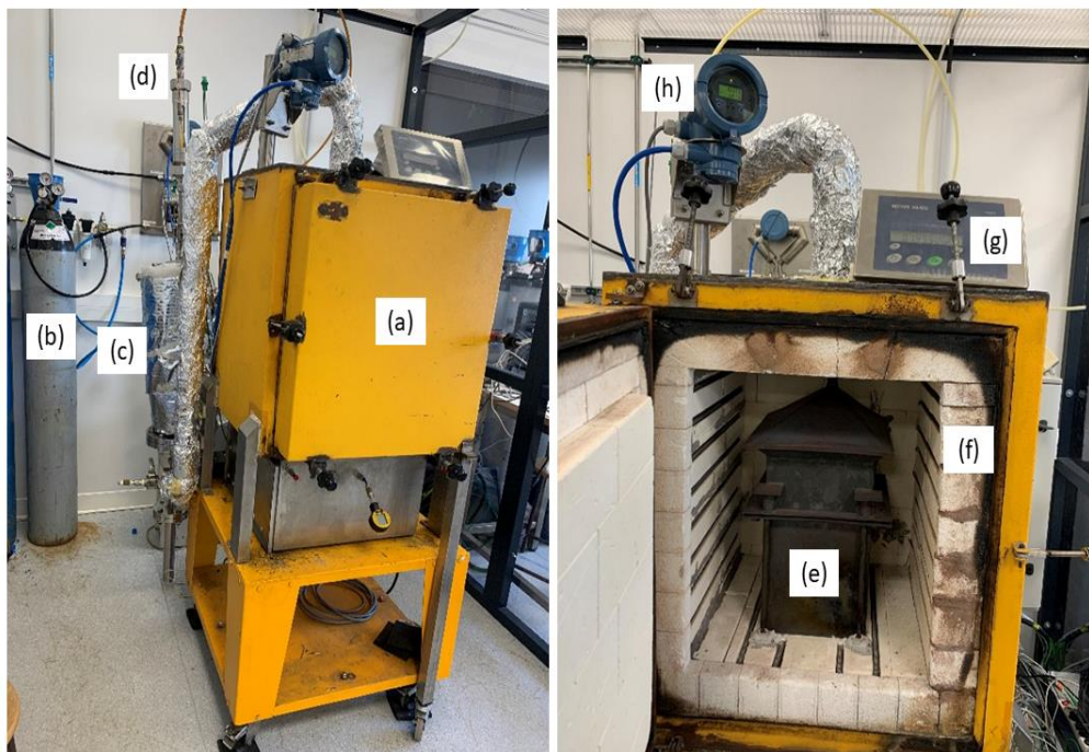
Figure 41: Experimental set-up of macro thermogravimetric reactor: (a) main reactor, (b) nitrogen gas supply, (c) condensation system, (d) filter and gases vent line, (e) pyrolysis basket, (f) muffle furnace, (g) sensitive balance, and (h) gas flowmeter.
