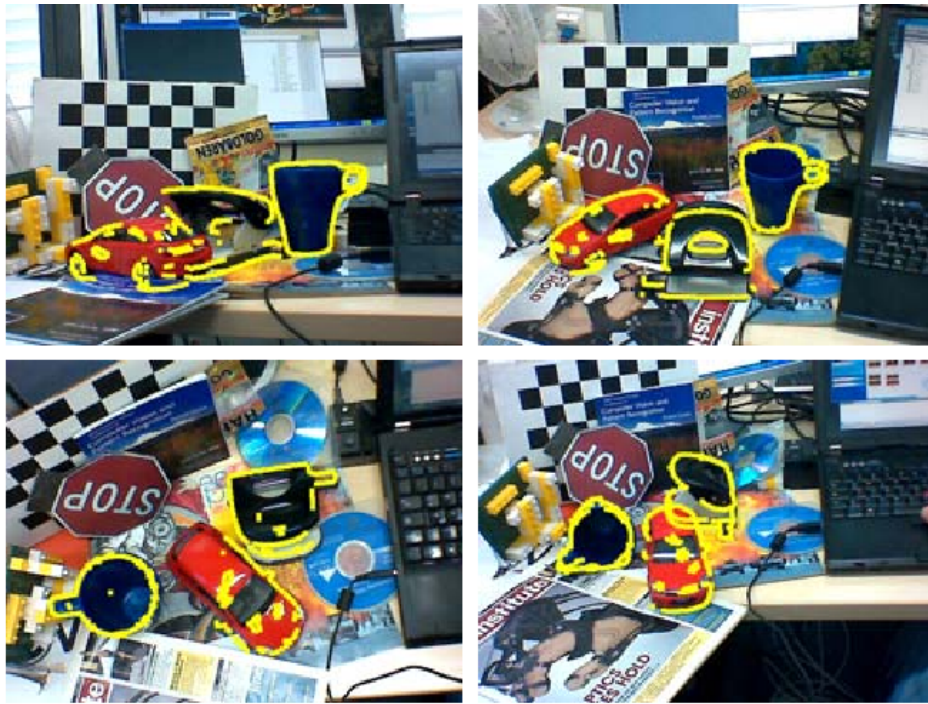
Figure 2.5: A method can detect texture-less 3D objects in real-time under different poses over heavily cluttered background using gradient orientation. Hinterstoisser et al. (2011)
