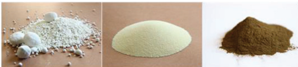
Figure 2: Different sources of feed grade ZnO. Powders vary in color, structure according to the manufactured process. Left to right, powder produced with different methods (1) French method, (2) hydrometallurgical and (3) American method.
