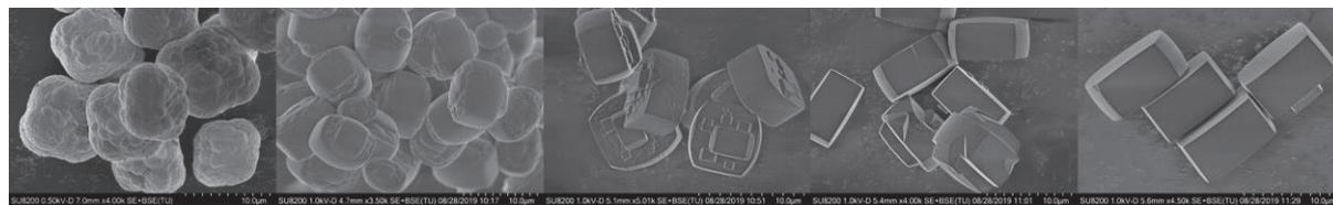
**Figure 1.** SEM images of the as-synthesized microporous ZSM-5 with Si/Al ratios of 25, 50, 100, 200 and infinite (from left to right).
