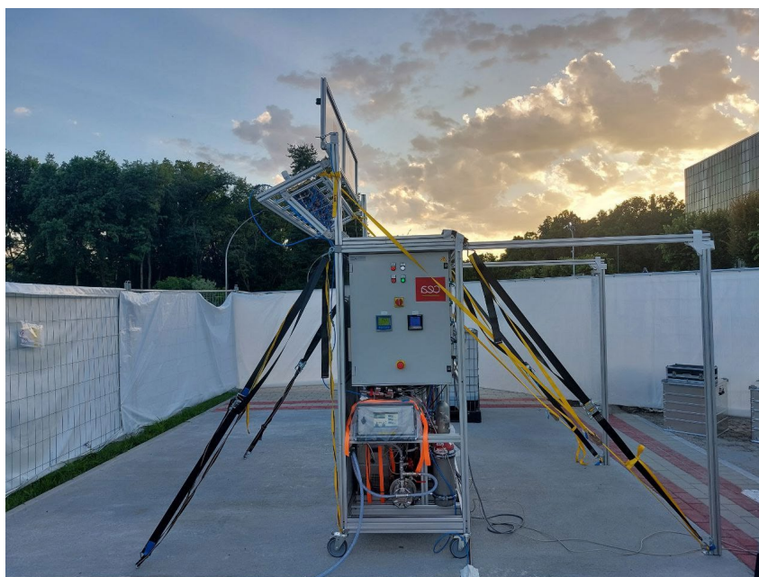
Figure 63. Top: Schematic view of the EASI Fuel device with IPEC modules in series and bioreactor; Bottom: Picture of the EASI Fuel device installed for a 3-day demonstration test at the JRC in Ispra in July 2022.
