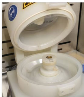
Figure 15. Fabrication of BiVO 4 photoanodes by sol-gel spin coating method.
