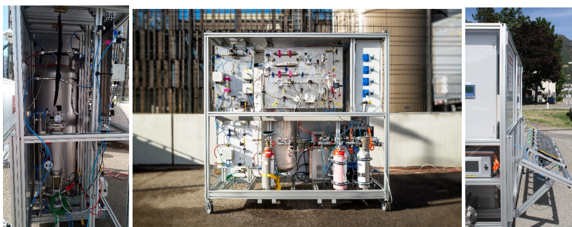
Figure 65. Left: side view of the EASI Fuel device showing the bioreactor in the front (see Figure 74 in Appendix for an enlargement) and the feed water tank in the back; Center: back view showing the control panel; Right : side view showing 4 of the 5 IPEC modules for solar \text{H}_2 production.
