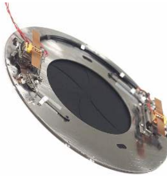
Figure B.5: An image of the VC1 Fast shutter comprising of 6 blades with a damage-threshold of 100 \text{ mW/mm}^2 .
