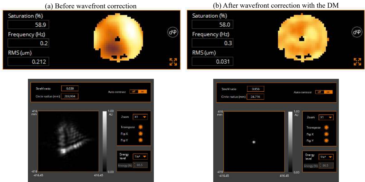
Figure B.9: Screenshots of wavefront measurements (top-panel) and the corresponding PSF (bottom-panel) without (a) and with (b) wavefront correction with the DM.
