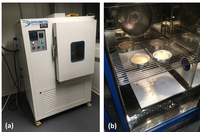
Figure 2.3.4: The conditioning in humidity uses a climatic chamber (a) set at a specific temperature and RH, in which samples are disposed (b) above aluminum-foil structures.
