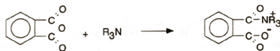
Figure 1.2.5: Example of possible initiation with a tertiary amine as catalyser resulting in an carboxylate ion
