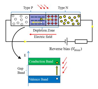
Figure 2.9: Light to electrical signal conversion in PD: energy diagram (bottom) and PN junction dynamics under a bias voltage.
