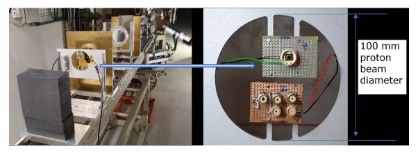
Figure 4.6: Left) CAL Proton beamline, including the QPD mounting. Right) Zoom on QPD mounting.
