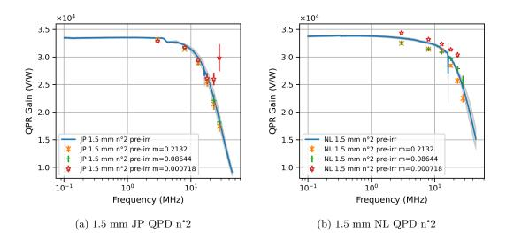
Figure 5.21: QPR gain from plotter and sweeper results versus the frequency for a) 1.5 mm JP QPD n°2 and b) 1.5 mm NL QPD n°2. Measurement performed at room temperature with  $V_{\text{bias}} = 5$  V for JP QPDs and  $V_{\text{bias}} = 30$  V for NL QPDs. Data points show the average QPR gain over the four QPR channels, and the error bars area shows the standard deviation between channels.
