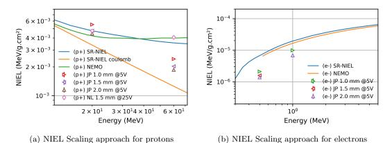
Figure 5.11: Relative comparison between the NIEL of InGaAs and the dark current experimental damage factors from a) JP and NL QPDs under 20 and 60 MeV protons and b) JP QPDs under 0.5 and 1.0 MeV electron. Data points show the average dark current over the four QPD segments.
