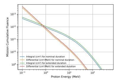
Figure 3.14: Mean cumulative solar proton flux spectra for the nominal LISA mission duration [41]. Based on this model, ESA has established the requirements for the InGaAs QPD, summarized
