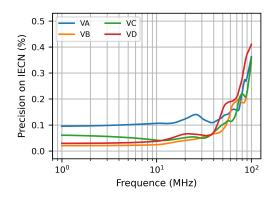
(a) Precision on the EICN measurement function of the frequency.
