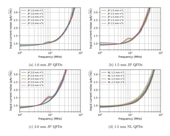
Figure 5.19: EICN versus frequency for a) 1.0 mm JP QPDs, b) 1.5 mm JP QPDs, c) 2.0 mm JP QPDs, and d) 1.5 mm NL QPDs, before irradiation performed at rooms temperature with  $V_{\rm bias} = 5$  V for JP QPDs and  $V_{\rm bias} = 30$  V for NL QPDs. Data points represent the average noise across four channels, processed via LOESS smoothing (detailed in Section 4.5). The grey-shaded area shows the standard deviation between segments.
