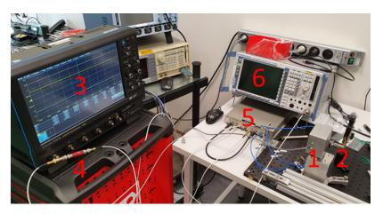
Figure 4.24: Picture of the QPR EICN measurement set-up: 1. QPR in a mechanical enclosure,2. White light source, 3. LECROY Oscilloscope, 4. Thorlabs EF500 DC Block, 5. Preamplifier, and Rohde and Schwartz Spectrum Analyzer.
