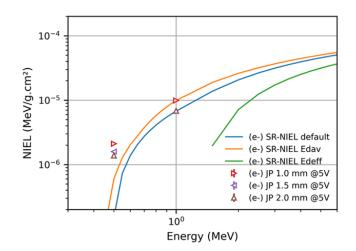
Figure 5.13: Relative comparison between new NIEL values for InGaAs and the dark current experimental damage factors from JP QPDs under 0.5 and 1.0 MeV electron. Data points show the average dark current over the four QPD segments.
