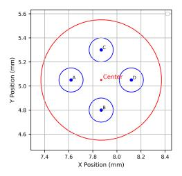
Figure 4.23: Illustration of the laser beam's relative alignment across the QPD's segments, using XYZ translation tables.
