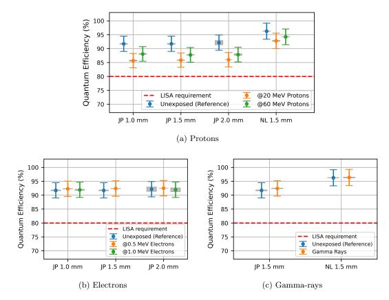
Figure 5.9: QE for a) JP and NL QPDs under 20 and 60 MeV, b) JP QPDs under 0.5 and 1.0 MeV electrons, and c) 1.5 mm JP and 1.5 mm NL QPD under gamma-rays performed at room temperature and 5 V for JP QPD and 20 V for NL QPD. Data points show the average dark current over the four QPD segments, and the grey-shaded area shows the standard deviation between segments. Error bars represent the measurement precision.
