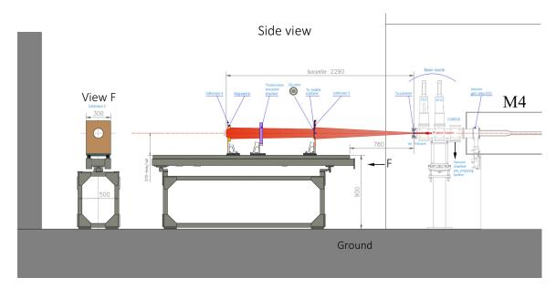
Figure 4.5: Side view of R&D irradiation room at CAL proton facility.
