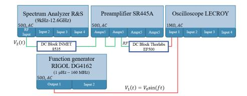
Figure 4.28: Electrical diagram of the EICN setup with QPR replaced by a wave generator.
