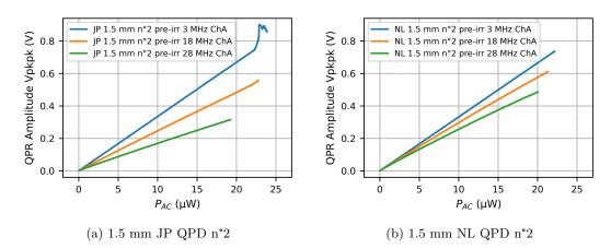
Figure 5.20: QPR output amplitude voltage at frequencies of f = 3, 18, and 28 MHz and m = 0.2132 versus the AC signal amplitude arriving on the a) 1.5 mm JP QPD n°2, and b) 1.5 mm NL QPD n°2. Measurement performed at room temperature with  $V_{\text{bias}} = 5$  V for JP QPDs and  $V_{\text{bias}} = 30$  V for NL QPDs.
