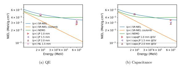
Figure 5.18: NIEL scaling approach applied to a) QE results for JP and NL QPDs, and b) Capacitance results from JP QPDs. Data points show the average damage factor over the four QPD segments.
