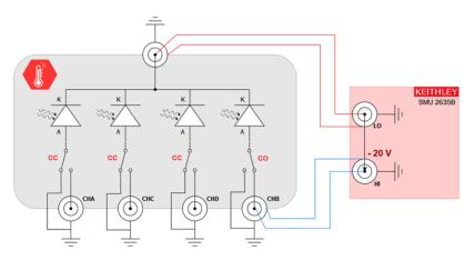
Figure 4.18: Electrical schematic of the QPD connection to the Keithley 2635B SMU.
