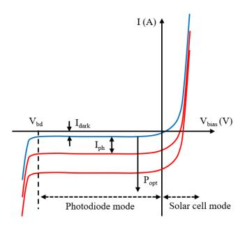
Figure 2.10: Output current of the PN junction in function of the  $V_{\text{bias}}$  applied. In blue correspond of the current with no incoming light ( $P_{opt} = 0$ ) and in red with  $P_{opt} > 0$  and increasing.
