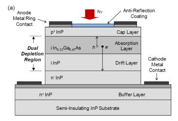
Figure 2.12: Ultra-fast InGaAs DDR PD structure [37].
