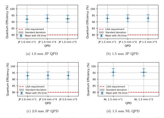
Figure 5.4: QE for a) 1.0 mm JP QPDs, b) 1.5 mm JP QPDs, c) 2.0 mm JP QPDs, and d) 1.5 mm NL QPDs. Data points show the average dark current over the four QPD segments, and the grey-shaded area shows the standard deviation between segments. Error bars represent the measurement precision. Measurements were performed in a clean room at a temperature of approximately  $25 \pm 1$  °C.
