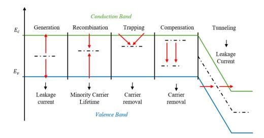
Figure 3.13: The five physical mechanisms created by crystal deflects in the semi-conductor.
