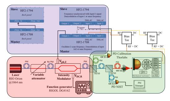
Figure 4.31: Diagram of the interferometric setup with red: LISA interferometric signal generation block, green: Signal monitoring and test module block, and blue: Control and acquisition block.
