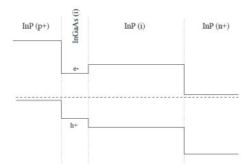
Figure 2.13: The basic InGaAs/InP heterojunction dual-depletion photodiode at zero bias [34].
