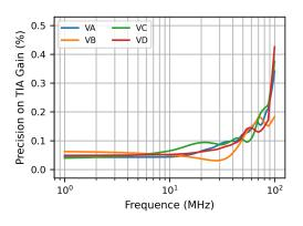
(b) Precision on the TIA Gain measurement function of the frequency
