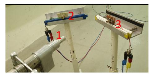
Figure 4.9: Picture of the QPD copper support in the void chamber.
