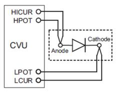
Figure 4.13: Four-point capacitance measurement configuration [106].
