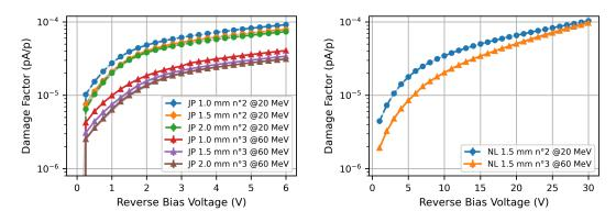
(a) Damage factor for JP QPDs under protons ir- (b) Damage factor for NL QPDs under protons irradiation radiation
