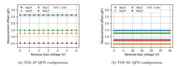
Figure 4.15: Measured stray capacitance for each channel under JP (a) and NL (b) QPD configurations, highlighting the setup's maximum stray capacitance at 2.63 pF at 6V.
