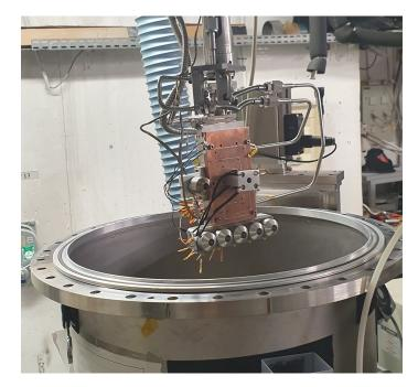
Figure 4.8: Picture of the QPD copper support in the void chamber.
