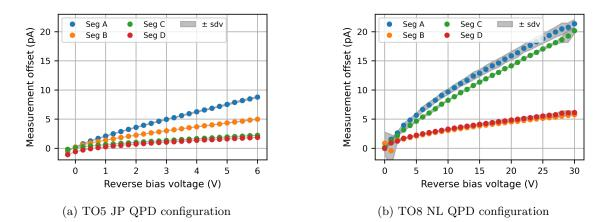
Figure 4.14: Measured stray currents for each SMU channel under JP (a) and NL (b) QPD configurations, highlighting the setup's maximum stray current of 21 pA at 30V.
