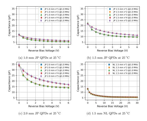
Figure 5.3: Capacitance versus bias voltage  $(V_{\text{bias}})$  for a) 1.0 mm JP QPDs, b) 1.5 mm JP QPDs, c) 2.0 mm JP QPDs, and d) 1.5 mm NL QPDs at 25 °C and 1 MHz. Data points show the average dark current over the four QPD segments, and the grey-shaded area shows the standard deviation between segments. Error bars represent the measurement precision.
