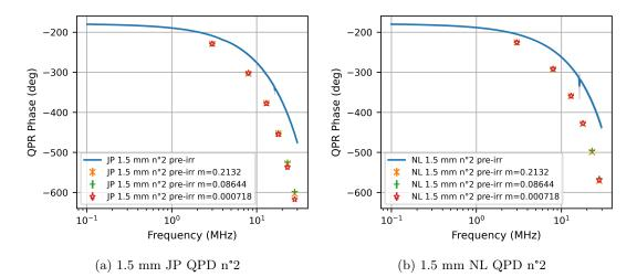
Figure 5.22: QPR phase response from plotter and sweeper results versus the frequency for a) 1.5 mm JP QPD n°2 and b) 1.5 mm NL QPD n°2. Measurement performed at room temperature with  $V_{\text{bias}} = 5$  V for JP QPDs and  $V_{\text{bias}} = 30$  V for NL QPDs. Data points show the average QPR phase response over the four QPR channels, and the error bars area shows the standard deviation between channels.
