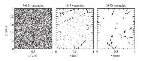
Figure 3.9: Initial distribution of vacancies produced by 10 MeV protons (left), 24 GeV protons (middle) and 1 MeV neutrons (right). The plots are projections over 1 µm of depth (z) and correspond to a fluence of  $1 \times 10^{14}$  cm<sup>2</sup> [58].
