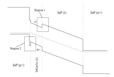
Figure 2.14: The basic dual-depletion diode under strong reverse bias voltage. Both the electrons and the holes have a barrier to overcome in order to reach the p+ and n+ electrodes [34].
