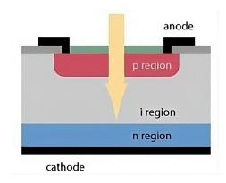
Figure 2.11: Cross-sectional view of a PIN PD.
