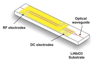
Figure 4.33: FIM principle schematics.
