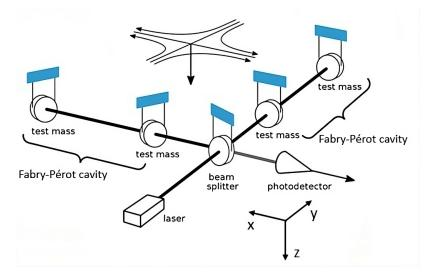
Figure 2.4: Simplified diagram of the LIGO detector [20].
