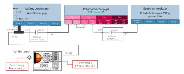
Figure 4.25: Electrical diagram of the QPR noise and TF experimental bench.
