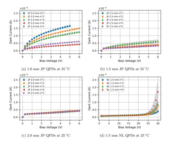
Figure 5.1: Dark Current versus bias voltage ( $V_{\text{bias}}$ ) for a) 1.0 mm JP QPDs, b) 1.5 mm JP QPDs, c) 2.0 mm JP QPDs, and d) 1.5 mm NL QPDs at 25 °C before irradiation. Data points show the average dark current over the four QPD segments, and the grey-shaded area shows the standard deviation. Error bars represent the measurement precision.
