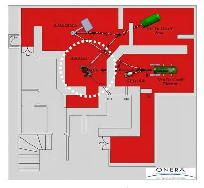
Figure 4.7: The accelerators and beam lines at ONERA (Mirage is highlighted with broken white line).
