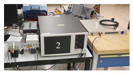
Figure 4.10: Images of the experimental setup for QPD dark current and capacitance measurements: (1) Metallic enclosure housing the QPD, (2) KEITHLEY measurement system, and (3) LTR-1200 temperature control unit.
