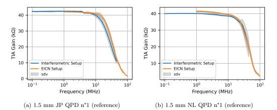
Figure 4.38: TIA gain results versus frequency, using a) 1.5 mm JP reference QPD, and b) 1.5 mm NL reference QPD, for both EICN and interferometric setups.
