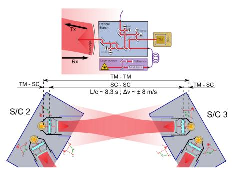
Figure 2.6: TM to TM measurement principle within a MOSA (top) and their combination to form a LISA link (bottom) [25].
