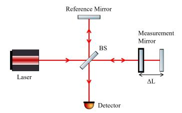
Figure 2.3: Schematic of the Michelson Interferometer.
