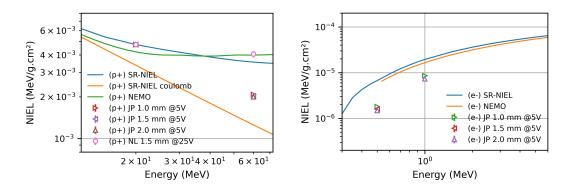
(a) Damage factor for JP QPDs under protons irradiation radiation radiation
