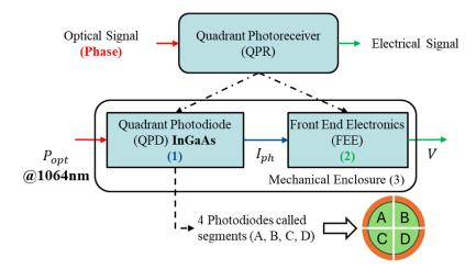
Figure 2.8: Schematic diagram of LISA QPR system with (1) the QPD, (2) the FEE, and (3) the mechanical enclosure.
