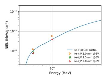
Figure 5.14: Relative comparison between NIEL values based on uniform distribution of  $E_d$  for InGaAs and the dark current experimental damage factors from JP QPDs under 0.5 and 1.0 MeV electron. Data points show the average dark current over the four QPD segments.
