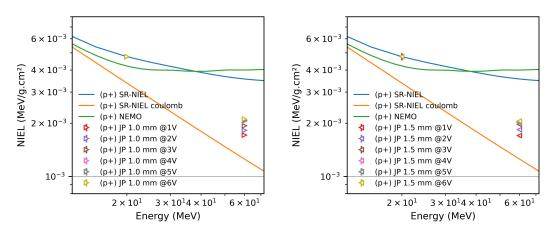
(a) Damage factor for JP QPDs under protons irradiation radiation radiation
