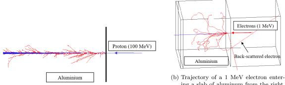
(a) Trajectory of a 100 MeV proton entering Aluminum from the right.
