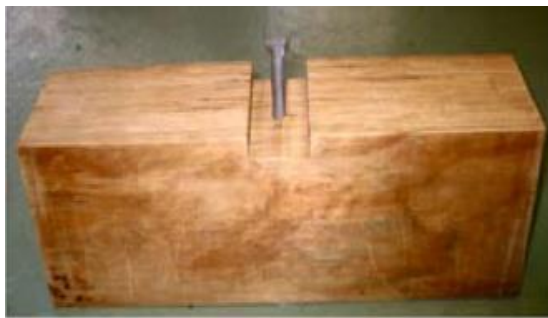
Fig. 1-27 Rectangular plug with screw, Deam et al. [65]
