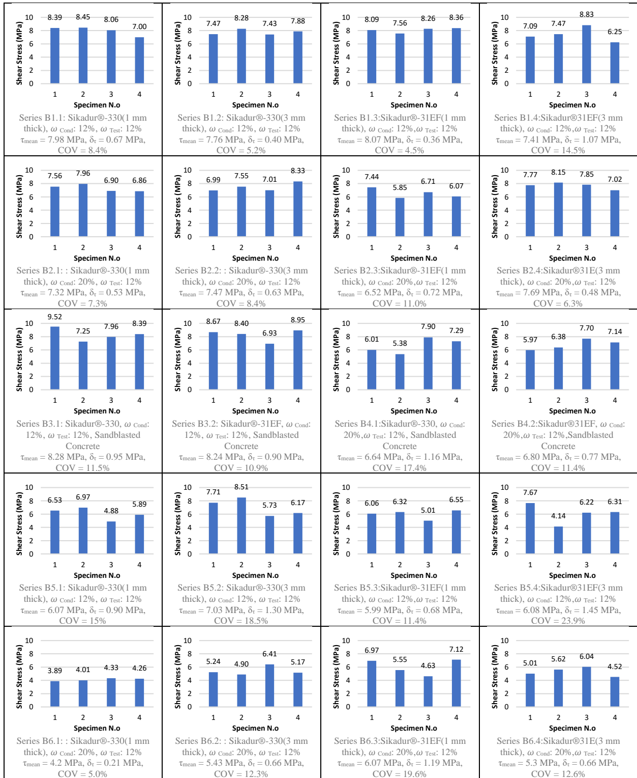
Fig. 2-11 Shear strength of all tested TCC specimens, (a) wet TCC joints, and (b) dry TCC joints
