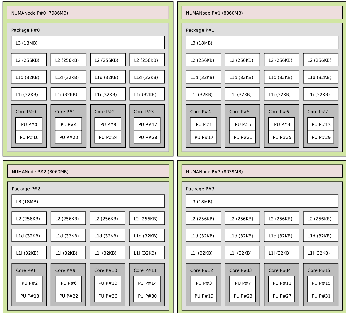
Figure 4.5: Mid-end host server: Dell PowerEdge R910 (Istopo picture)
