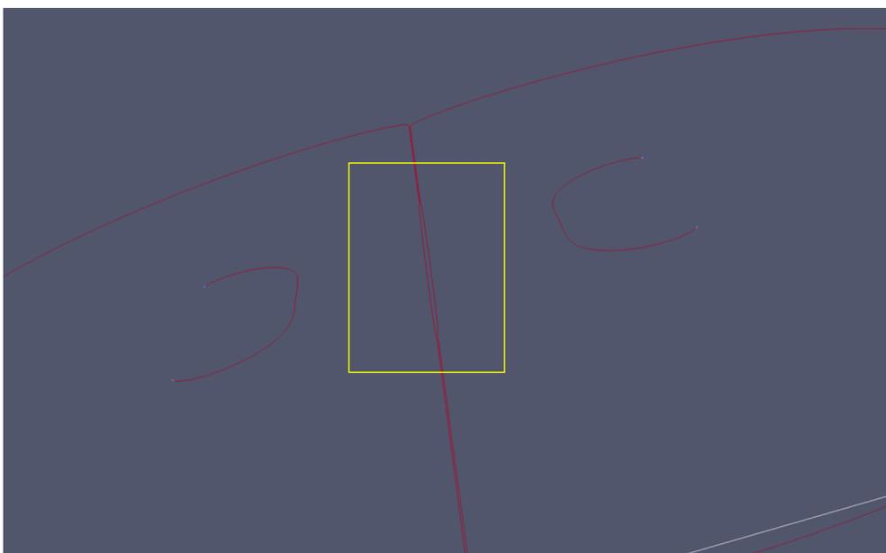
Figure 6.6: The separation of a dipole (shown in the yellow rectangle), the shear stress applied at this moment is the strength of the dipole
