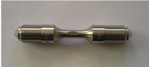
(a) The A316L stainless steel specimen used for the EBSD scan.
