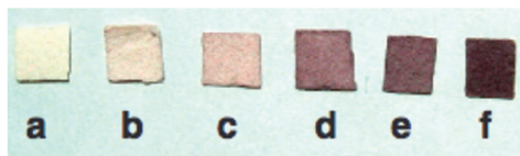
Figure 36 : Calibration de la concentration de la solution de vanadium ; a = 0 mg/L -> f = 50 mg/L. [75]
