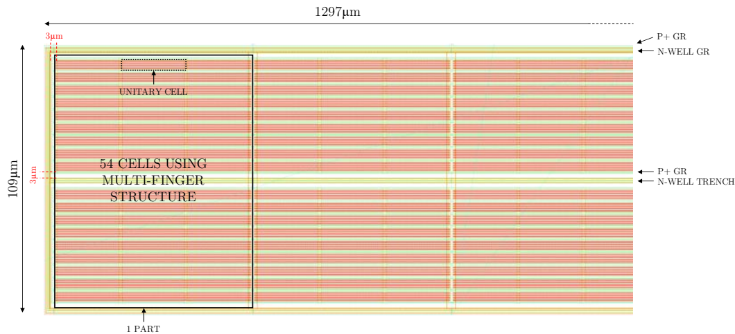
Figure 3.14 – Layout of the switching element. For easy readability, only few cells are illustrated without the metal routing.
