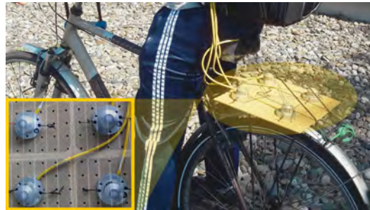
Figure 2.22: Photo of our biking measurement trip, carried out from 10h34 to 11h22 on the 21/06/2021 in Toulouse, France. The positioning of the pyranometers was inspired by how the four PV modules could be positioned.
