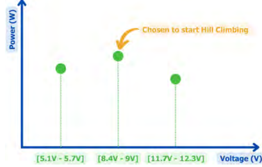
Figure 3.19: The general idea of our proposed simple GMPPT algorithm.
