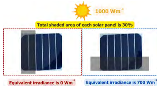
Figure 2.10: Equivalent irradiance received by the PV module when being proportionally shaded the same (30%) but the shading patterns are different.
