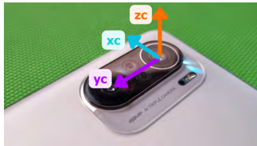
Figure 1.12: Visualization of how the camera coordinate reference is oriented relative to the phone's camera.
