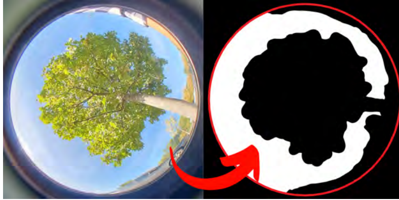
Figure 1.5: A simple example of a horizon that is impossible to describe using PVGIS horizon tool.
