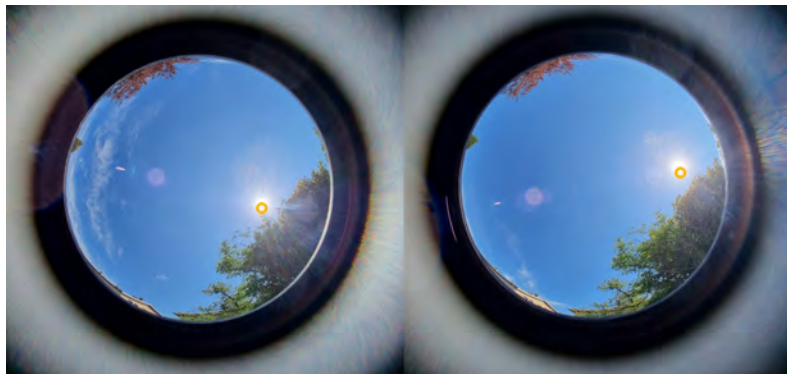
Figure 1.24: Example of two solar position evaluation photos. The yellow circle marks where our program estimates the sun to be in our image.
