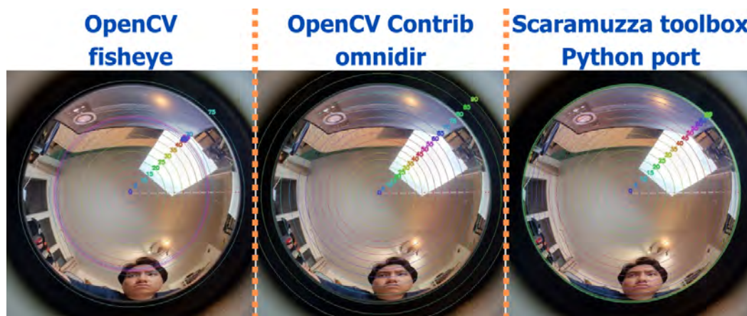
Figure 1.18: Protractor’s photo with remapped angles overlaid to evaluate the precision of three calibration libraries tested.
