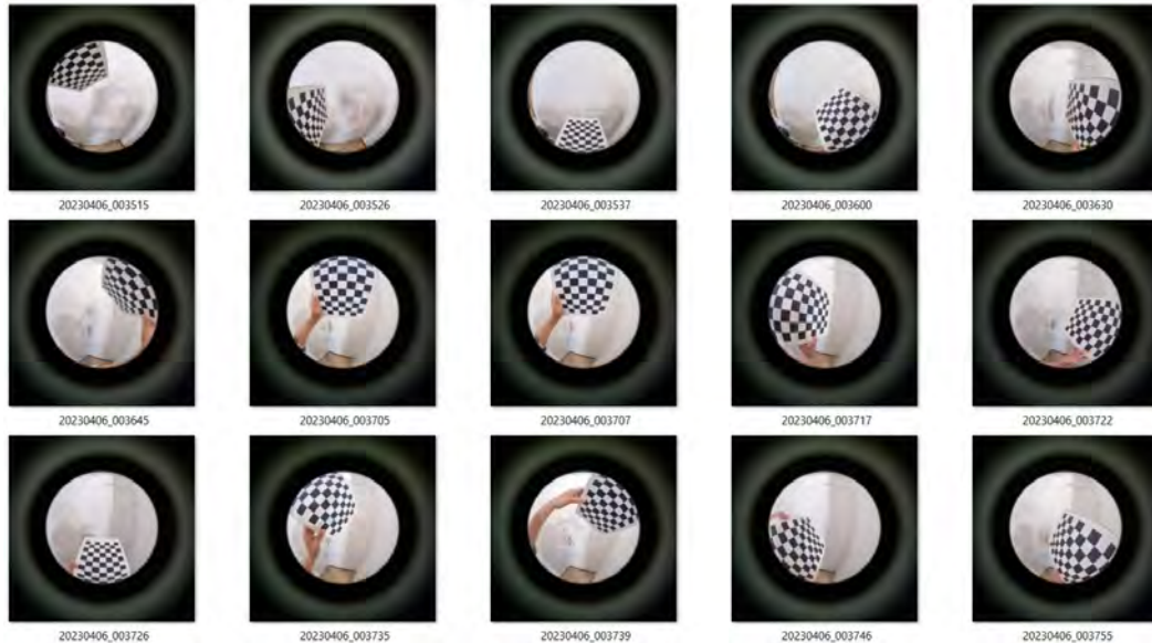
(a) Example of a good calibration image set. All images are properly taken and we have the pattern covers the entire camera's FOV.
