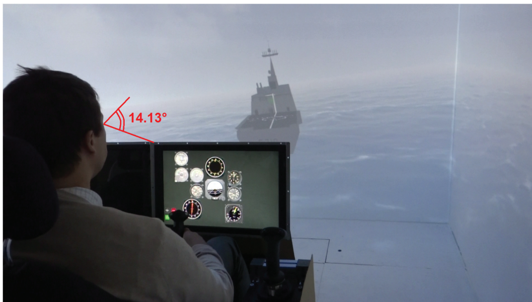
Figure 1. Expert pilot performing an Astern approach. The outside-the-cockpit downward field of view was limited to 14.13° below the eye level. The ground projection also allows the pilot to see partially on his side the scene below the helicopter.
