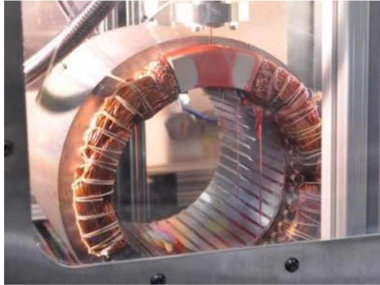
Figure 24. The experiment of Bennion film flow over end winding [57]
