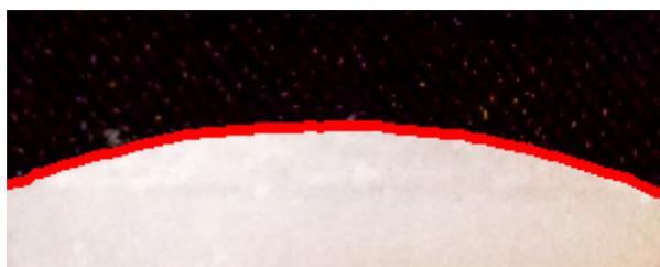
(b) A stimulus (Shore 00-10  $R=21.4$  mm) with edge detected, bolded, and highlighted in red color for visualization.
