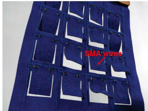
(a) SMA wires behind louvers can be heated to curve to open/close them to change the *Porosity* for adjusting daylight incidence [72].
