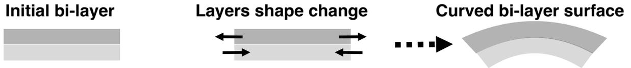
(a) Bi-layer cylindrical surface with Zero Gaussian *Curvature*: when two layers change their *Length* in a parallel direction, the bi-layer structure will form a cylindrical surface bending toward the relatively shorter layer. For example, as shown in this Figure, with the upper layer increasing its *Length* and the bottom layer decreasing its *Length*, it will bend toward the bottom layer.
