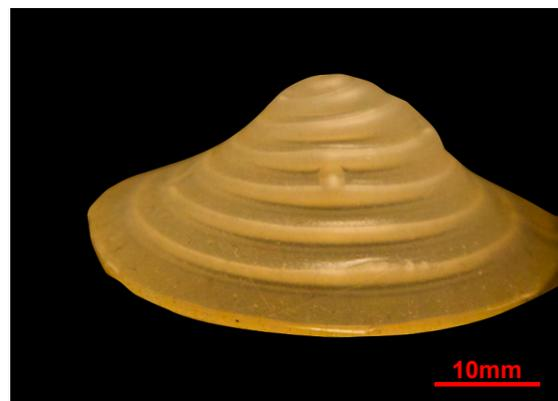
(d) The Baromorph inflates with an inner air pressure of 12 Psi. We can see that the membrane covering air channels stretch in the center more than in the edge. This leads to the inflated Baromorph having a larger slope in the center than in the edge.
