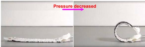
(c) An elastomer tube sewn in fabric and fiberglass bi-layer structure curves to elastomer side when deflated [530].
