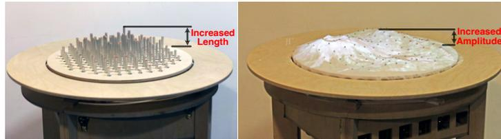
(b) An uncovered matrix of actuated pins (Left) can be covered with a piece of fabric (Right) to transform the *Length* change of pins into *Amplitude* change of the fabric surface.
