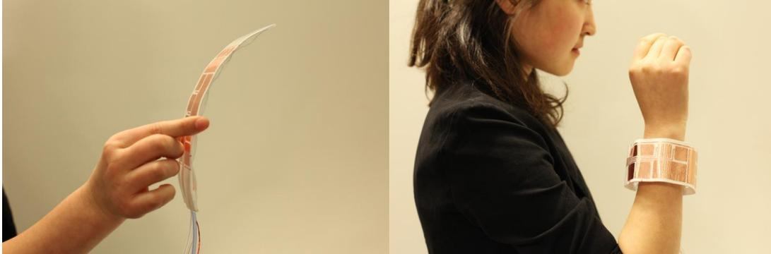
(a) A phone adapting its shape to different tasks. For example, it can transform into a wristband (right) to be worn [509].
