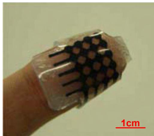
(b) A matrix of dielectric elastomer membranes, with a density of 3 actuated *Amplitude*-changing units per  $cm^2$  (20 actuated elastomer bladders over  $1.54\text{ cm}^2$ ) [234].
