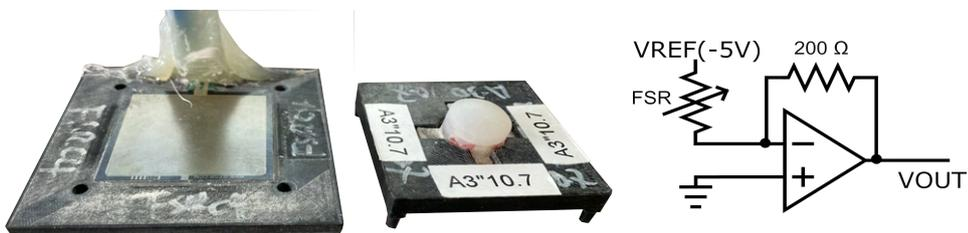
(d) (Left) The pressure sensor Interlink FSR406 stuck on the 3D printed support and (middle) a stimulus to install on this support. (Right) The schematics of the circuit for one sensor.
