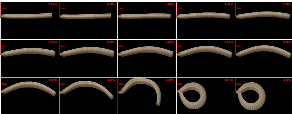
(c) Photos of *Closure* changing prototype under different air pressures.
