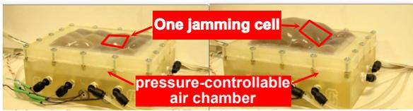
(a) **Pneumatically inflating + Jamming:** A matrix of jamming cells was added on the top of a pressure-controllable chamber. Before jamming, the matrix of cells can be bent with increasing pressure in the chamber, and each cell can be jammed to become rigid [418]
