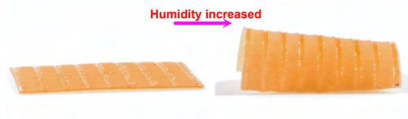
(h) A gelatin bi-layer structure curves to more porous gelatin side when humidity is increased [476].
