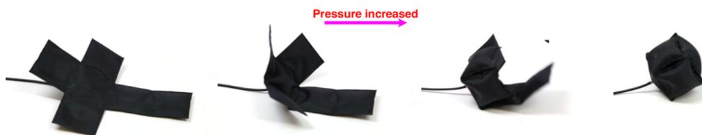
(b) A non-stretchable fabric airbags and fabric bi-layer structure in the form of a polyhedron net can inflate to curve, creating a closed polyhedron with *Closure* changing from 0% to 100% [318].
