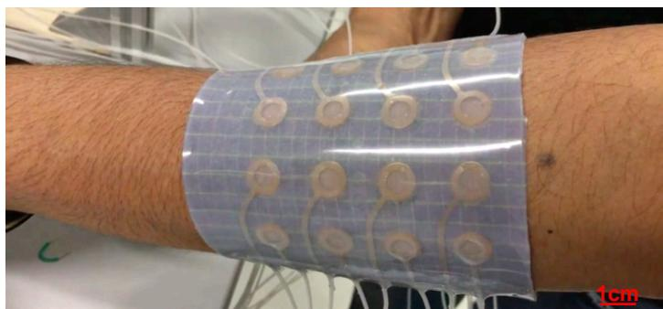
(c) A matrix of inflatable elastomer bladders, with a density of 0.19 actuated *Amplitude*-changing units per  $cm^2$  (16 actuated elastomer bladders over  $84\text{ cm}^2$ ) [412, 466].
