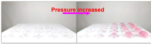
(a) Elastomer bladders can inflate into spherical balloon-like shapes with their *Volume* increasing [119].
