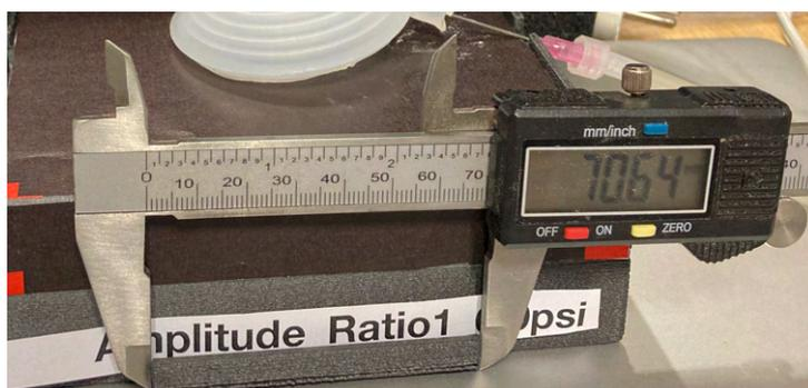
(b) A vernier scale measuring the label holder's length to ensure the precision of the conversion between pixels and mm.
