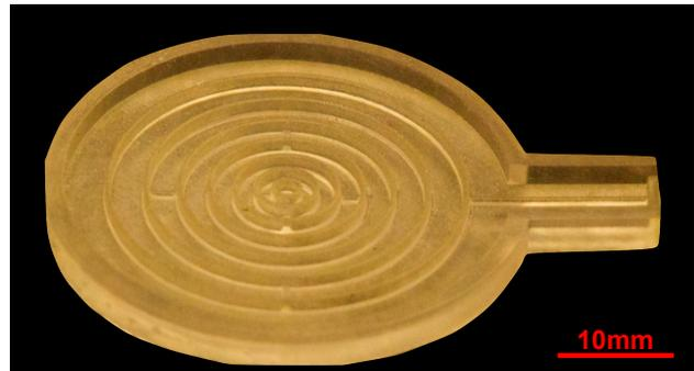
(b) A Baromorph mold 3D printed with a Form3 high precision Stereolithography (SLA) 3D printer [109] in clear resin [368].
