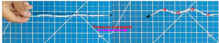
(a) Four rigid pieces (white colors in figure) prevent an elastomer tube with sheath's extension underneath them, leading to its curving in 4 parts and increases its *Zero-crossing* points from 0 to 4 [225].
