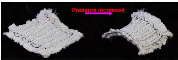
(c) Two orthogonally placed pneumatically extendable elastomer sewn in fabric layers form a saddle shape when two layers inflated together [530].
