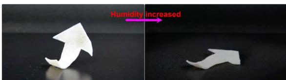
(i) An hydrogel and fabric bi-layer structure curves to hydrogel side when humidity is increased [371].
