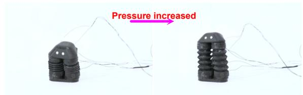
(d) Elastomer bladders molded into bellows-like shape can inflate to increase their *Length* [300].
