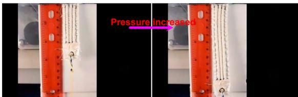
(e) Elastomer tubes sewn into fabric with limited radial expansion can inflate to increase their *Length* [530].
