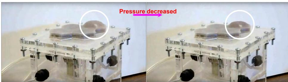
(b) The four pentagonal prisms in this figure are elastomer bladders with ground coffee, whose air inside can be independently vacuumed out (jammed) to increased *Strength* respectively. The cylinder in the white circle (left) is pushed to be a dome shape by the air chamber below it before being jammed and then vacuumed to be jammed (right). The force needed to process it back to flat depends on the vacuum level inside it [416].
