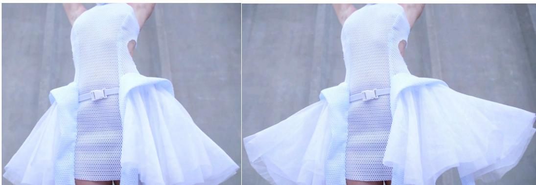
(d) Hedonic and symbolic purposes: A dress can expand (Left to Right) to protect the wearer and signal others to maintain a distance when a proximity sensor detects intrusion into personal space [498].
