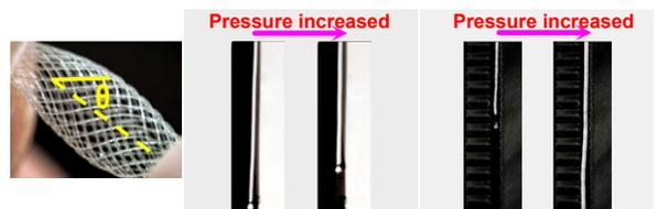
(f) Elastomer tubes with non-stretchable filaments braided around to limit its radial expansion can inflate to decrease (Middle) or increase (Right) their *Length* respectively to different braiding angles (Left) [225].
