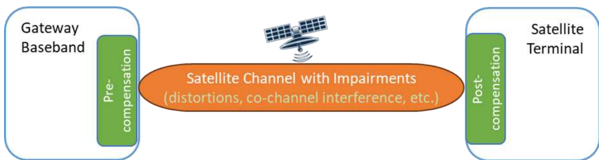
Figure 3.1: Forward link pre-compensation and post-compensation in satellite systems
