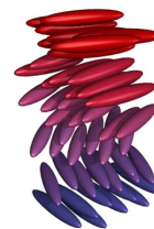
Figure 1.29: Schematic representation of the CNCs arrangement in the cholesteric liquid crystal phase. Reproduced from [Barrett, 2021].
