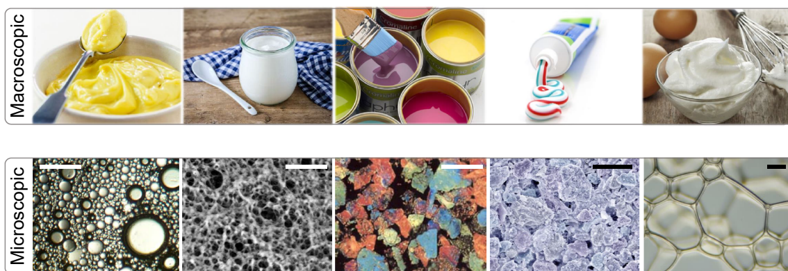
Figure 1.1: Examples of soft materials at the macroscopic scale (upper row) and at the microscopic scale (lower row). From left to right: mayonnaise, yogurt, paint, toothpaste, beaten egg whites. The scale bars on the upper corner of the microstructure images correspond to 150\ \mu\text{m} . Adapted from [Dagès, 2021].
