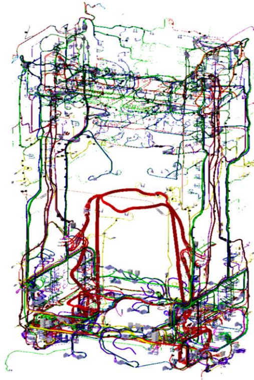
Figure 1.5 – 3D view of the harness bundles in a large telecom satellite.
