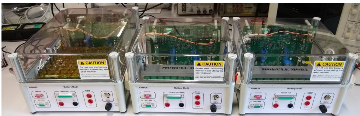
Figure 5.6 – MOBI prototypes with power and data interfaces visible on the front face.
