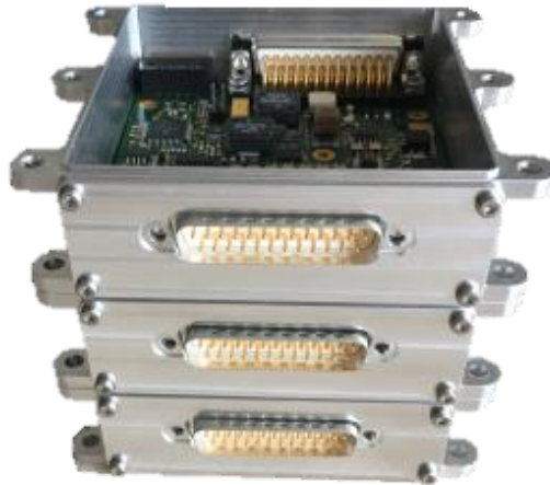
Figure 5.3 – Stacked BOMO-Cs rear panel with specific interfaces.
