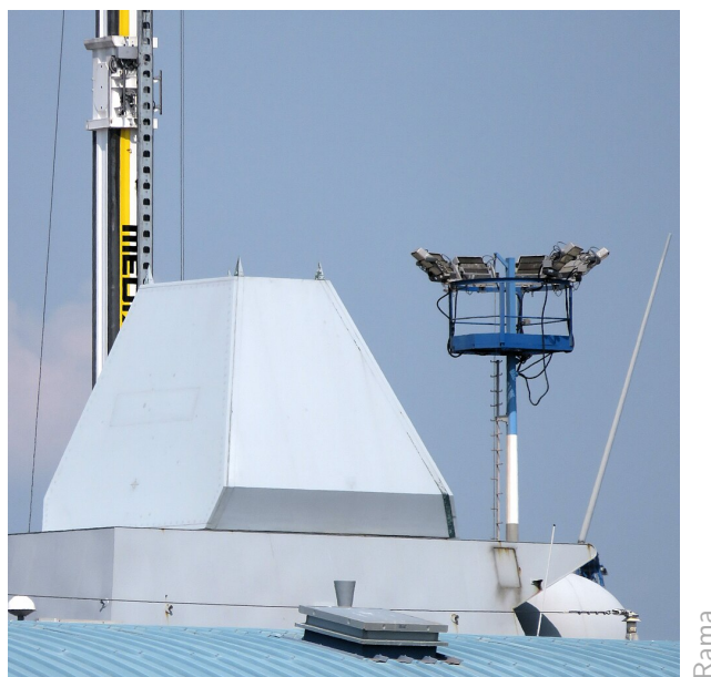
FIGURE B.1 – Radar Herakles.
