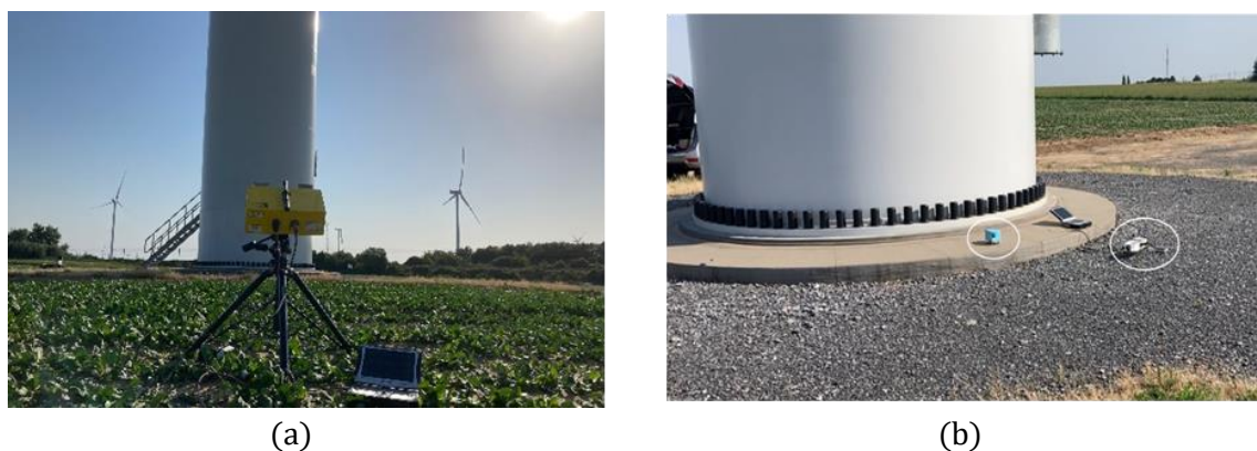
Figure 3-13: (a) The interferometry radar, (b) The geophone instruments.
