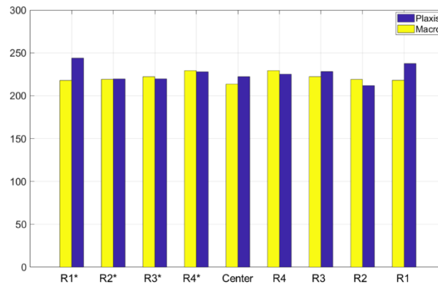
Figure 5-20: Maximum axial load along the line of RIs aligned with the wind direction, under the self-weight.
