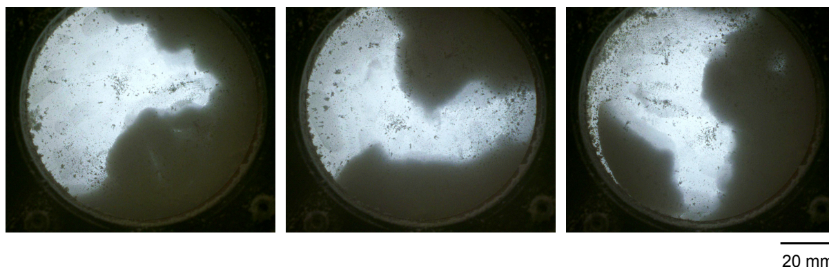
Figure 7: Illustration of the ice aggregates formed inside the drum with three individual pictures of the IP-A sample at 143 K. The aggregates are of centimetre-size, hard to break with just a fall in the drum, and no flowing behaviour is observed at this point.
