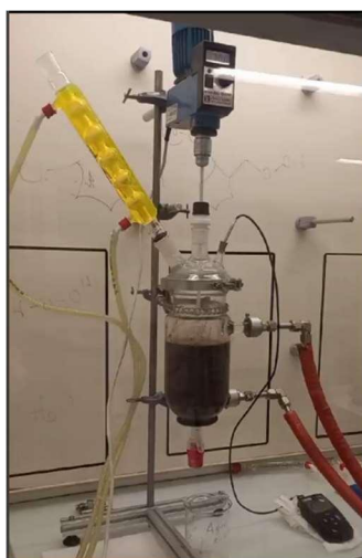
Figure II-7: Experimental set-up for hemicellulose extraction from biomass.
