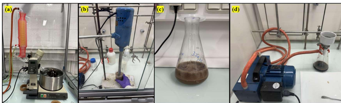
Figure II-8: Separation of lignin from hydrolysate. (a) Elimination of formic acid by rotative evaporator; (b) precipitation of lignin by Ultra-Turrax type “rotor/stator” disperser; (c) settling of lignin in the hydrolysate; (d) separation of lignin from hydrolysate.
