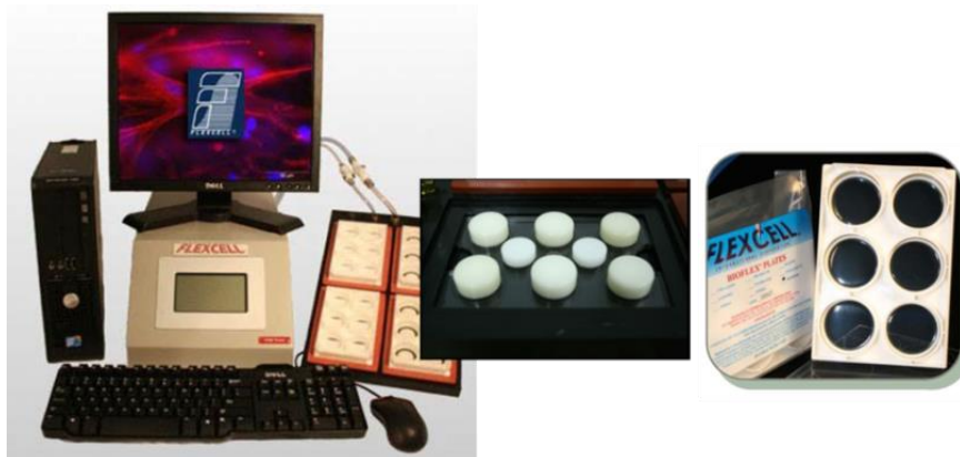
Figure 32: Illustration of Flexcell® FX 5000™ Tension System
