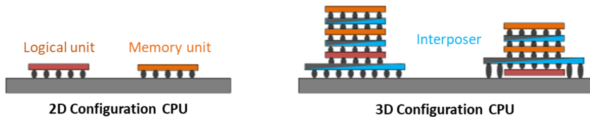
Figure 0. 2D and 3D configurations for microelectronics components.
