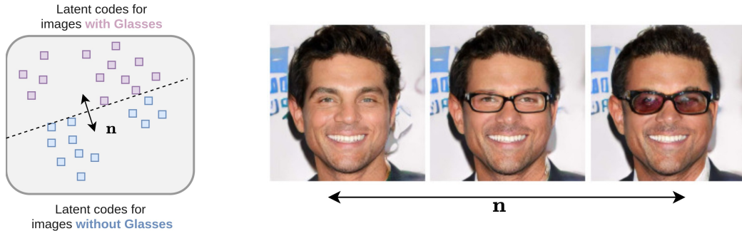
Figure 3.1: Extracting a semantic direction using the decision boundary of a binary classifier. (a) \mathbf{n} is the vector orthogonal to the decision boundary (dotted line) of a ‘glasses’ latent classifier. (b) Translating the latent code with \mathbf{n} leads to adding glasses that become more visible as the magnitude of the translation increases. Figure taken from [127].
