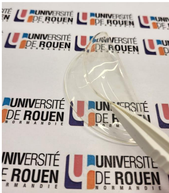
Figure 5.17. Image of obtained composite CAB/[DETA][BUPH] 29 membrane.
