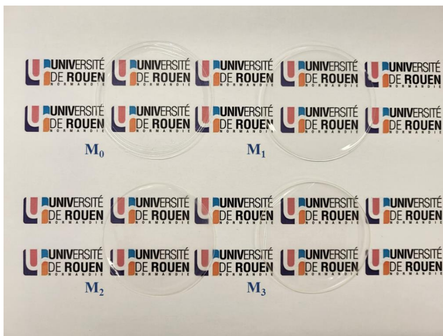
Figure 5.19. Images of obtained composite CAB/[DETA][TFS]-[DEPA][BUPH] membranes.
