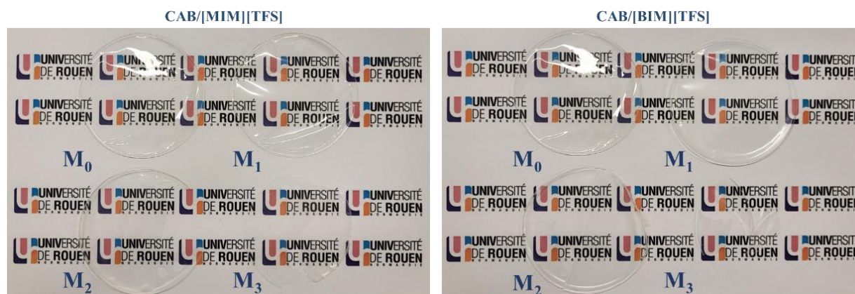
Figure 5.12. Images of obtained composite CAB/Pr-IL membranes.
