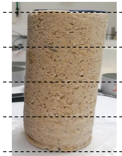
Figure 3.14 Frozen post-suffusion specimen
