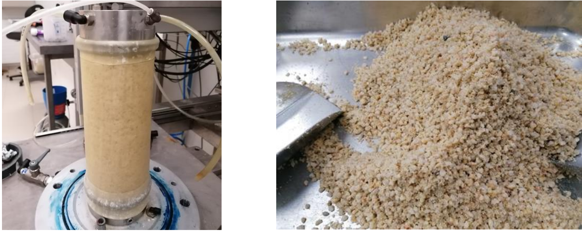
Figure 3.11 [a] Specimen positioning under bottom pedestal and [b] Gap Graded Palvadeau soil
