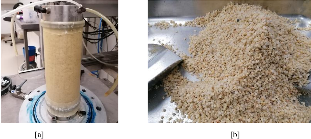
Figure 3.11 [a] Specimen positioning under bottom pedestal and [b] Gap Graded Palvadeau soil
