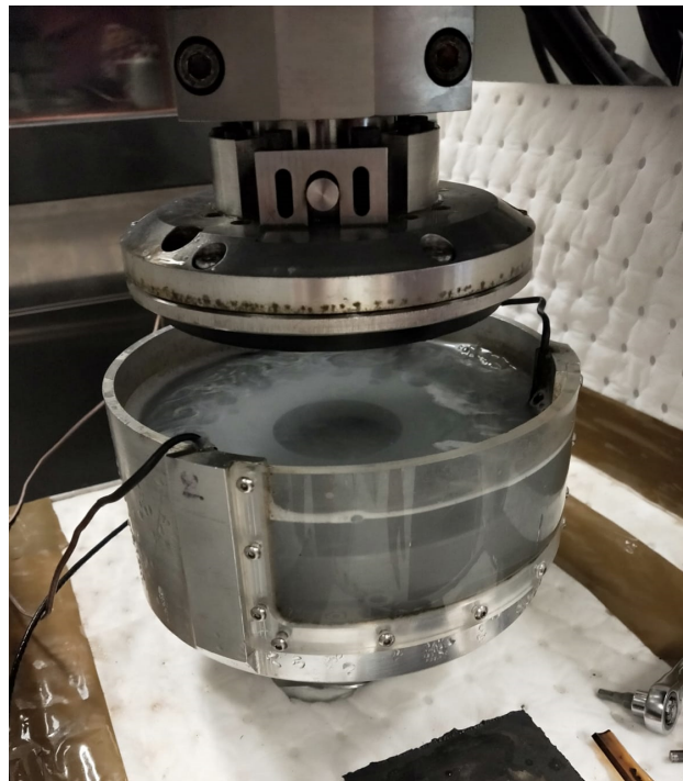
Figure 6.4: Substrate submerged inside a water tank attached to the Fixed Head support.
