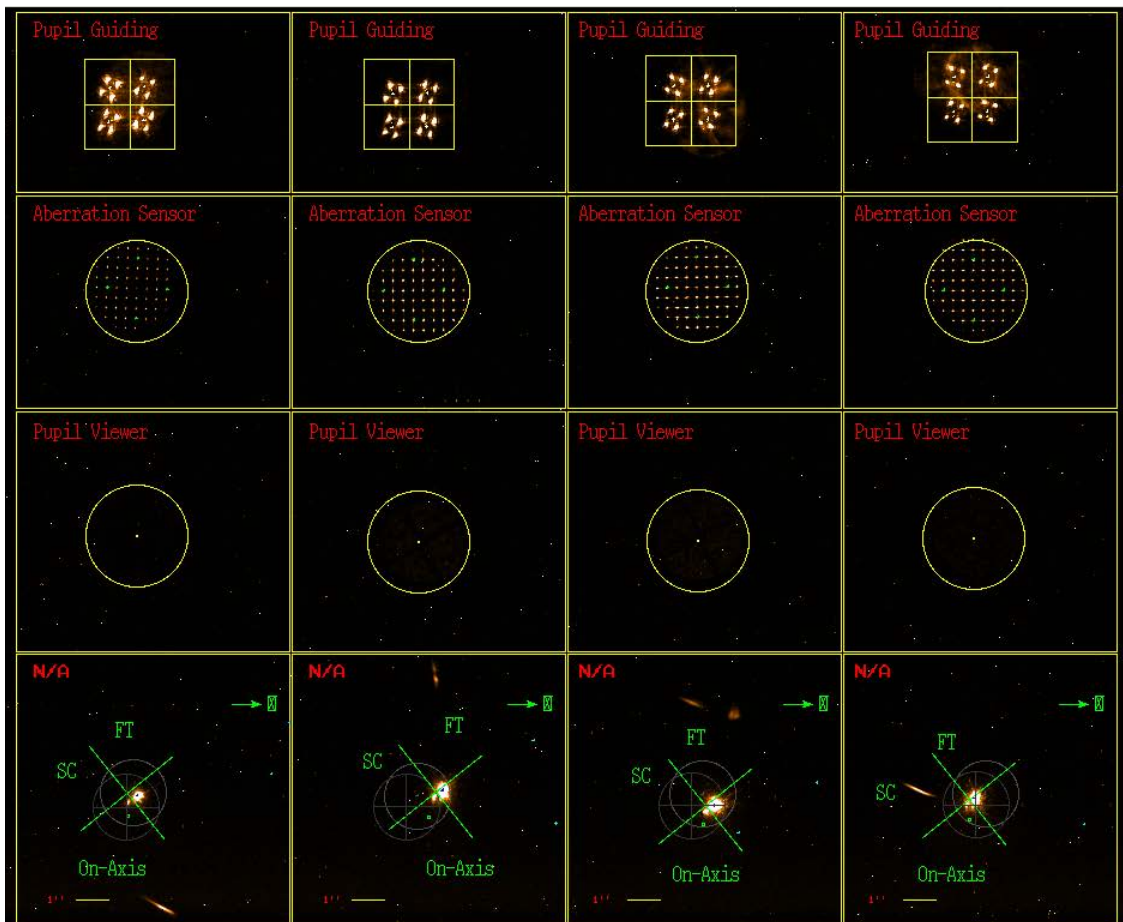
Figure 2.10 – Real-time display of the GRAVITY acquisition camera. Each column corresponds to one telescope. Vertical lines from top to bottom is: pupil beacons, internal Shack-Hartmann wavefront sensor, pupil viewer, and field image (From Anugu, 2016)
