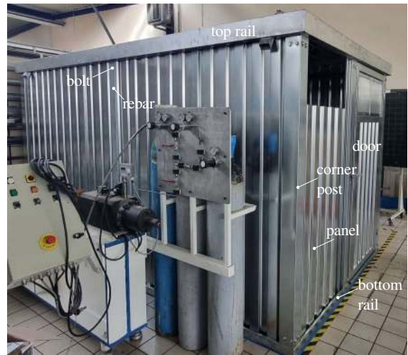
(b) Container cabin installed
