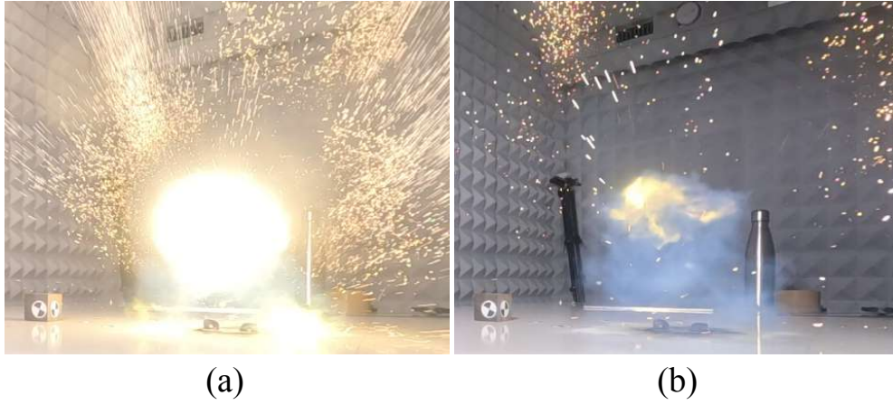
Figure 2.8: Explosion of exploding wire with spherical light at time t = 12.5 ms (a), and the dust produced at t = 25 ms (b), the images are captured by using GoPro11 with 240 fps and resolution 2704 \times 1520 pixels.
