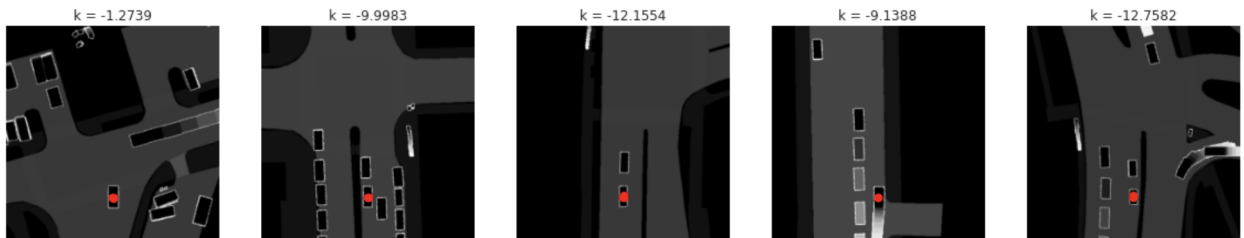
Figure 5.6: Examples of nuScenes stationary trajectories. Stationary trajectories, numerous in nuScenes, are discarded during training as they don't provide much value and can skew the evaluation metrics, especially accuracy as they are "easy examples". For discovery, we also discard them due to their irrelevance to the task at hand.
