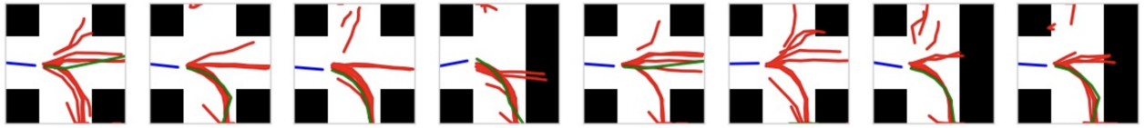
Figure 5.3: Left-going trajectories with an independent selection function. Trajectories generated by the “zero-point” model, exhibiting the capability of finding left trajectories but generating many degenerate trajectories in the process.
